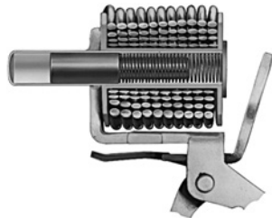
Overload Subsides Before Core Reaches Pole Piece
